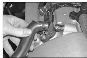
18. Remove the crankcase vent hose from the valve cover.
