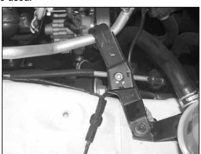
13. Rotate the A/C mounting bracket onto the power steering reservoir, then secure it using the bolt from the previous step. Tighten the A/C mounting nut.
