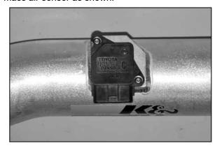
22. Secure the mass air sensor to the K&N® intake tube using the provided bolts as shown.
