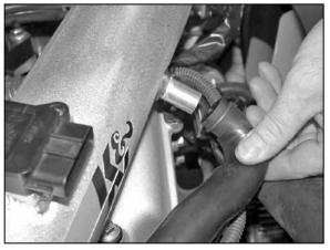
28. Connect the factory crankcase vent hose onto the K&N® intake tube as shown.
