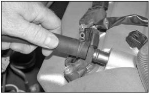
19. Flip the crankcase vent hose around and reconnect the opposite end of the hose to the valve cover
