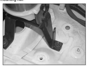
14. Remove the 12mm bolt that retains the power steering reservoir to the vehicle, then mount the provided bracket (07158) onto the vehicle with the bolt that was removed.
