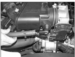
8. Remove the crankcase vent hose from the airbox as shown.
