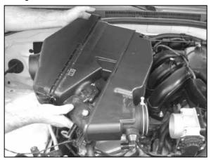
11. Remove the airbox assembly from engine as shown
