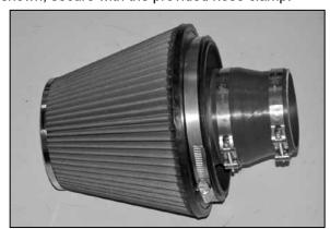
30. Install the provided silicone hose (084055) onto the filter adapter and secure with the provided hose clamp as shown.
