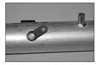
25. Install the tube mounting bracket (07133) onto the  $K\&N^{\circ}$  intake tube as shown.
