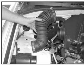
5. Remove intake tube from vehicle as shown.
