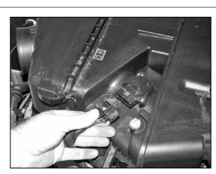
7. Disconnect the two mass air wire harnesses retaining clips from the airbox, then disconnect the mass air sensor electrical connection.
