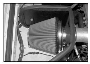
31. Install the air filter assembly onto the K&N® intake tube and secure with the provided hose clamp.
