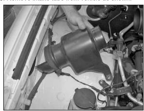
6. Remove the two bolts that secure the resonator to the inner fender, then remove resonator from vehicle as shown.
