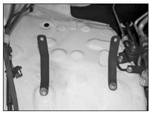
15. Mount the two provided brackets onto the vehicle with the provided hardware.
